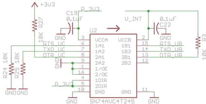
Since u-blox module's communication interface operates at 1.8VDC, while the STM32F205RGT6 microcontroller operates at 3.3VDC, we need voltage translators in-between them. This is achieved with two [SN74AUC4T245](#) non-inverting buffers. The default state of the USART pins is set with the help of pull-up and pull-down resistors, and the unused input pins are tied to GND.
