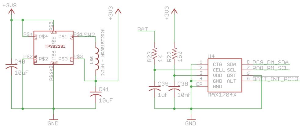
The output (3.8V net) of the PMIC is fed directly to the u-blox cellular module and a 3.3VDC high efficiency switching regulator ([TPS62290](#)). This 3.3VDC regulator helps power the microcontroller, fuel gauge and the buffers.
