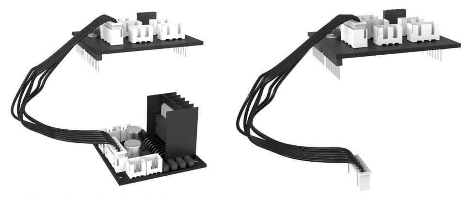
Connect the L298N board to V5 board.
