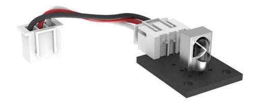
Connect the infrared receirer medule to the expansion board with the DuPont lines.
