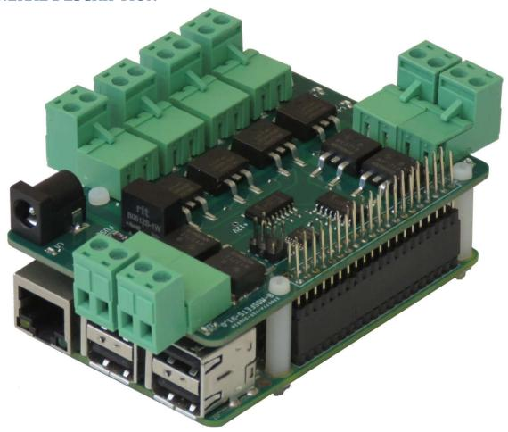
The 8-MOSFETS card is a stackable expansion card for Raspberry Pi. The card is compatible with all Raspberry Pi versions from Zero to 4. It offers a compact and inexpensive solution for adding up to 64 MOSFETs to your Raspberry Pi project.
