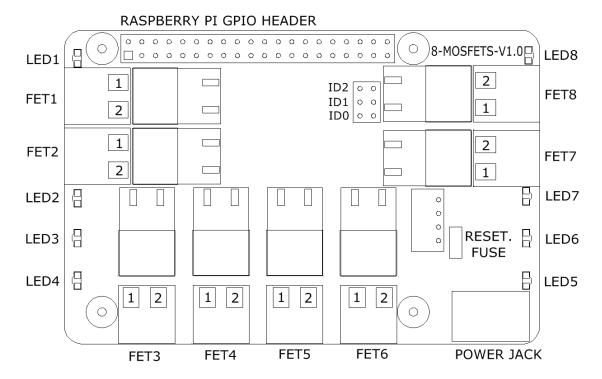
Your 8-MOSFETS card comes with appropriate mounting hardware. Up to eight 8-MOSFETS cards can be stacked on top of one Raspberry Pi.
