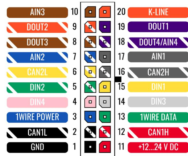
Figure 2 FMB640 Pinout
