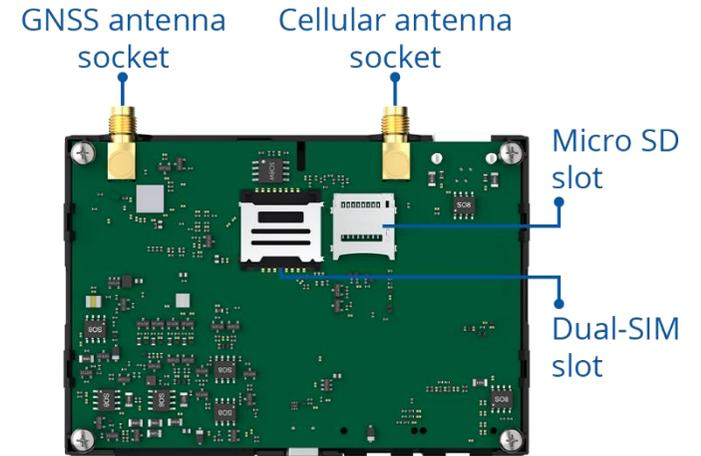
Figure 1 FMB640 device view
