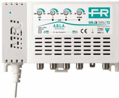
3-input (III+DAB, UHF, UHF) multiband TV indoor amplifier with 32dB gain and up to 120dB $\mu$ V output level on UHF band, separate amplification with independent level adjustment (20dB) for each input and low noise figure. T2 technology with UHF cut band for LTE 4G @790MHz and 5G @694MHz.
