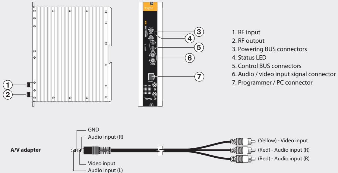
The modulator accepts audio and video inputs and modulates them according to the standard, into an IF of 38.9 MHz.
