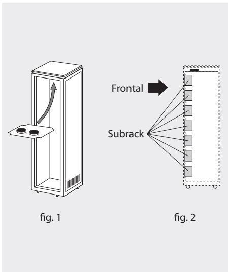
These ventilators will be installed on a tray that is fixed inside the cabinet (fig. 1 & 2). This way, the ventilators will force the fresh air entering from the base of the cabinet, to circulate between the modules and be expelled through a gap on top of the cabinet (3-5 cm approx.). See fig. 3.
