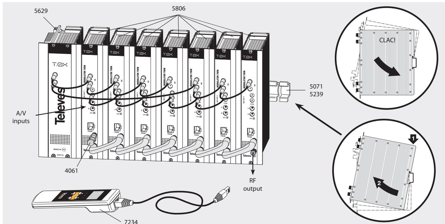
**NOTE:** The use of both PSU power outputs is recommended to balance the consumption. For example, 4+3 or 3+4
